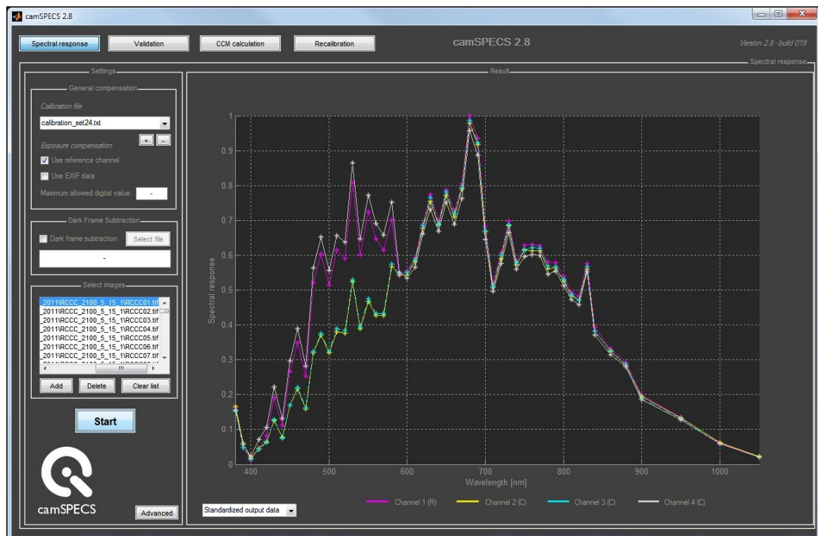
Figure 4: Spectral response of a non-standard color filter array: R-C-C-C
